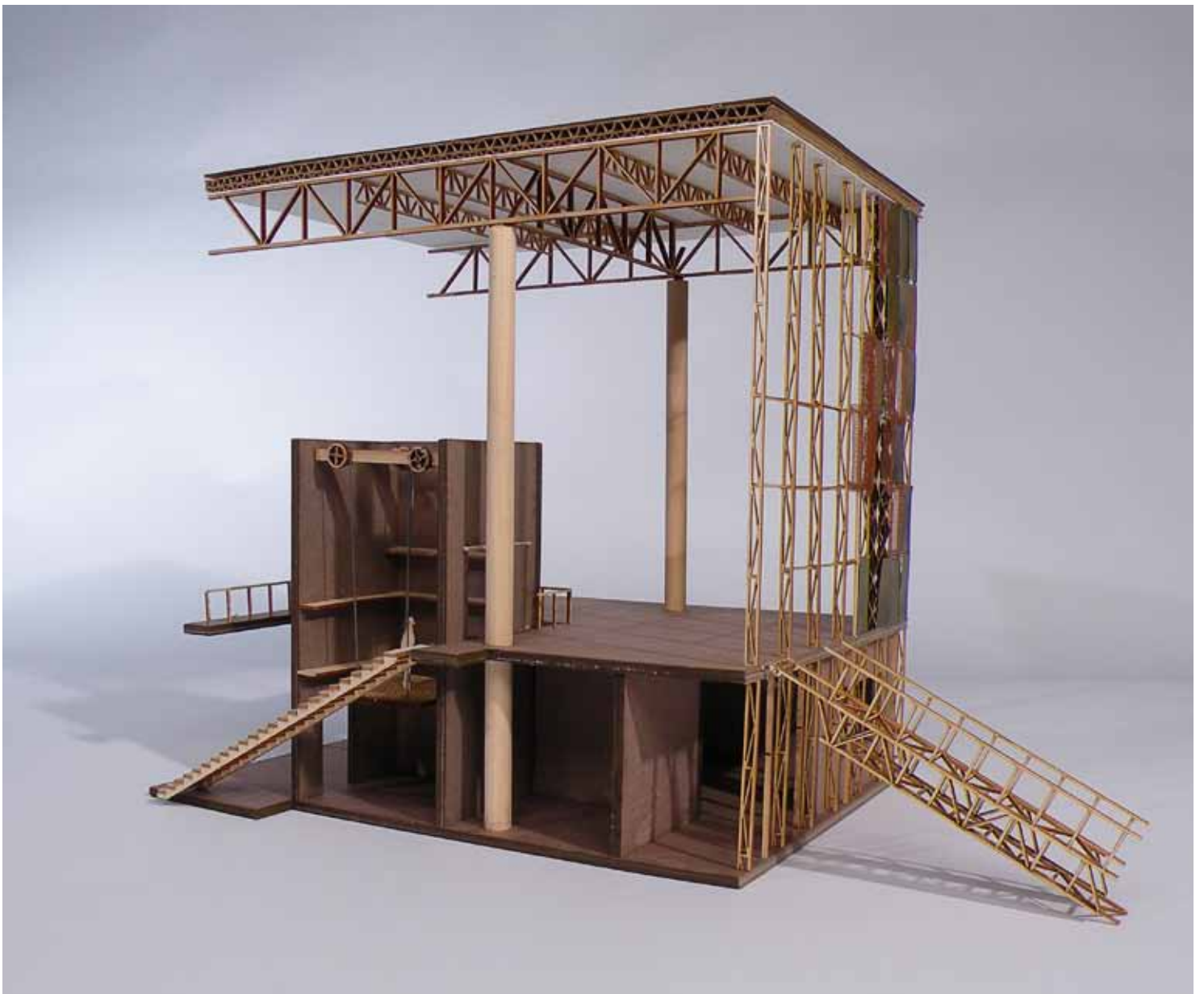
From Top to Bottom: Riparian Wetland Research & Learning Center model, 1/16'' = 1' . Section model of main building at vertical circulation and bridge to floating labs, 1/4'' = 1' .
